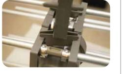
Step 12 Use two C-screws (14) to fasten together the overlapping ends of the plastic director supports (5).
